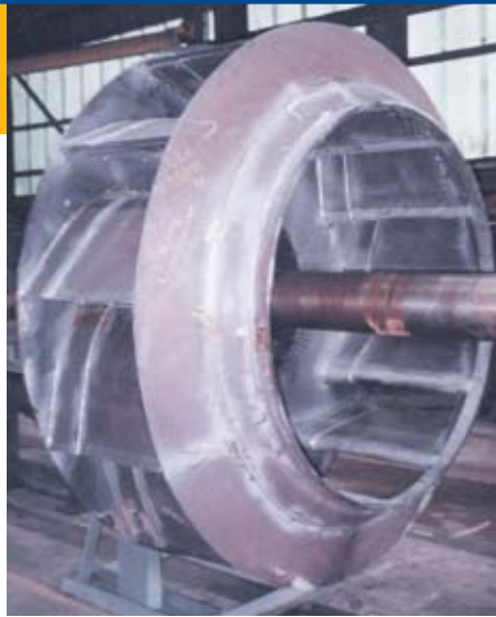
Rebuilt rotor assembly at the Birmingham plant.
